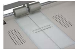
Centerline Registration with Vacuum Pumps
